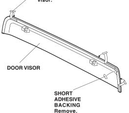
Push the two door visor brackets onto the door sash.
