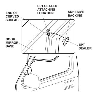
4. Trial fit the door visor to the door, and note the position that the EPT sealer needs to be installed in to seal and prevent wind noise. Remove the door visor. Remove the adhesive backing from the EPT sealer and attach it to the door mirror base as shown.
