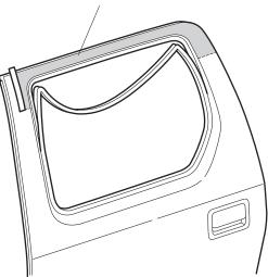
13. Attach masking tape to the ends of the long adhesive backings, and remove 2 to 3 in. (5 to 8 cm) of adhesive backings. Fold back the ends, and tape the ends to the front of the door visor. Remove the short adhesive backing.
